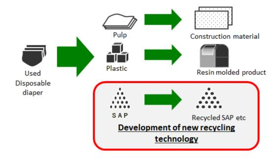
The recycling process for used disposable diapers used to face the challenge that SAPs, which would be swollen from absorbing urine, reduced the recovery rate of paper pulp, or even if SAPs were recovered, they were difficult to reuse because of the significant decrease in performance.
